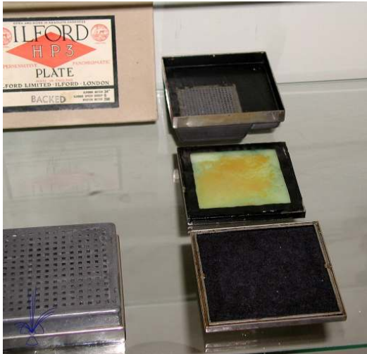
The first scintillation camera with collimator developed by Sven Johansson and Bengt Skanse. A photographic film was placed directly on the sodium-iodide crystal.
